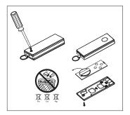
To replace battery for optional remote control transmitters - E943M, E940M & E945M, use a screwdriver blade to pry open the case as shown. Insert battery positive side up.
