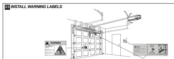
Three warning labels are provided with this opener: attach as indicated in the fig 1.
