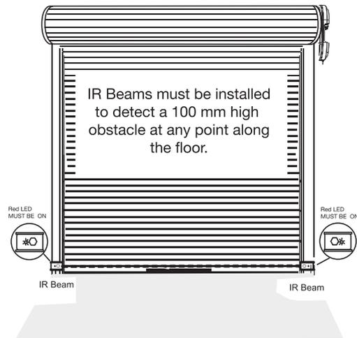
**ENABLING THE PROTECTOR SYSTEM:** (Factory default – IR beams are not enabled.)
